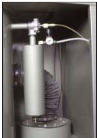
An independently adjustable pulse regulator maximizes cartridge-cleaning effectiveness and minimizes noise.
